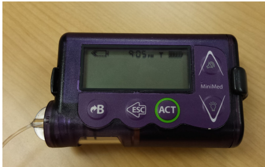
Insulin pump from medtronic that communicates wirelessly with continuous glucose monitor and traditional glucometer.
